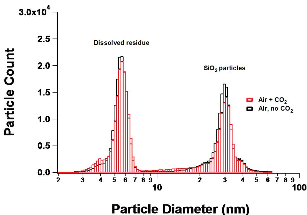
**Figure 1.** Particle size distribution of SiO<sub>2</sub> standard using air with and without CO<sub>2</sub>. The SiO<sub>2</sub> particles were accurately sized at 28.9 nm. A residue peak was observed at 5.5 nm due to soluble impurities. The results with and without CO<sub>2</sub> were similar. (Air flow = 1.5 L/min; CO<sub>2</sub> flow = 0.1 or 0 L/min).
