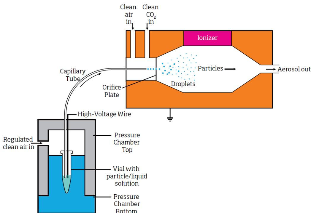
The EAG is used to generate a variety of nanoparticle and macromolecular aerosols for calibration, research, and quality-control applications. The use of air and CO<sub>2</sub> may not be suitable for air-sensitive samples. Therefore, the EAG was operated using nitrogen (N<sub>2</sub>) in place of air, and the CO<sub>2</sub> flow was varied, to determine the limits of EAG operation using N<sub>2</sub> and CO<sub>2</sub>.
