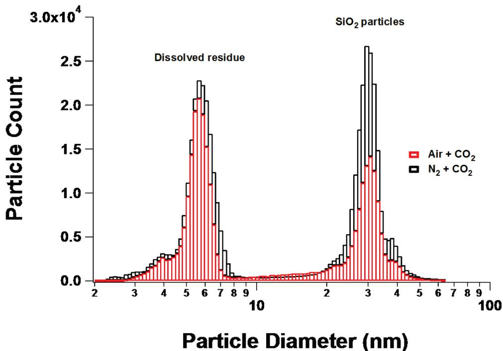
**Figure 2.** Particle size distribution of SiO<sub>2</sub> standard using air and N<sub>2</sub> with CO<sub>2</sub> at the nominal flow rate. The SiO<sub>2</sub> particles were accurately sized at 28.9 nm in both gases. The size of the residue particles was consistent in both gases. The SiO<sub>2</sub> particle count was higher using N<sub>2</sub>, while the particle count for the residue was similar in both gases. (Air flow = N<sub>2</sub> flow = 1.5 L/min; CO<sub>2</sub> flow = 0.1 L/min).
