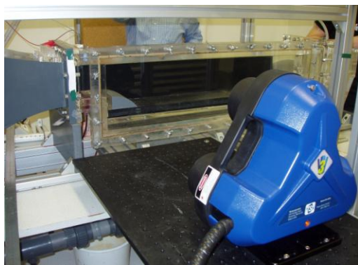
Fig. 2: Experimental setup showing the position of the 3D camera in relation to the measurement volume. The laser cone entered the water tunnel from the top.
