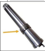
12. Attach the inlet to the column.
