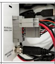
Attach the two smaller (white) connectors to the Power/ Communication inputs (J1 and J2) of the heated inlet control module.
