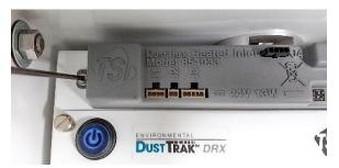
2. Push out elastic plug and install RH/Temp Sensor sealing gland. Removable nut should be installed on the inside of the enclosure.
