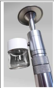
13. Install O-ring and route cable through the mounting ring. Pull excess cable through to prevent pinching of cable when inlet column is installed.
