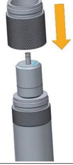
10. Install the O-ring into the bottom of the inlet.
