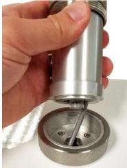
Carefully pull the Heated Inlet cable and connector through the slot in the Mounting Ring.
