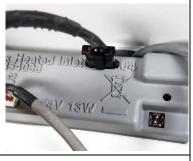
19. If using a Thiamis 1000 Node, route the other side of the cable to the power input on the Thiamis node (green connector). If you are not using the Thiamis 1000 telemetry node, this cable can remain disconnected.
