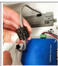
Carefully pull the Heated Inlet Assembly up.
