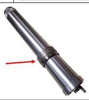
12. Attach the inlet to the column.
