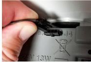
3. Remove the Ferrite Clamp Assembly. Note that the clamp is released by inserting and twisting a small flat blade screwdriver. Also, for purposes of re-assembly, note that the cable twists two times through the Ferrite.
