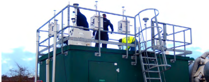
TSI's EDTPM2.5M, EDTPM10M and EDTDRXM were compared against European Reference Method Samplers, identified as PM10 and PM2.5 SEQ 47/50 manufactured by Sven Leckel GmbH.
