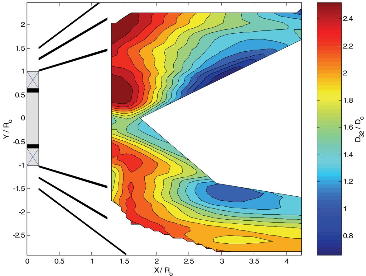
**Figure 2:** Measured Sauter Mean Diameter (normalized) for an operating gas turbine engine combustor.
