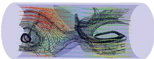
Streamlines indicating flow direction during the closed phase inside an artificial deformable silicone polymer heart valve.
