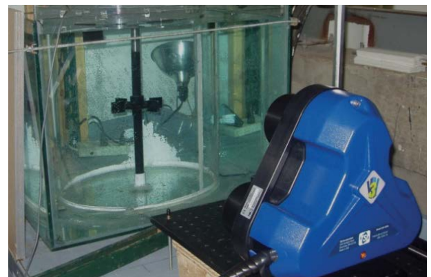
Experimental setup showing V3V™ system camera and Rushton Turbine.
