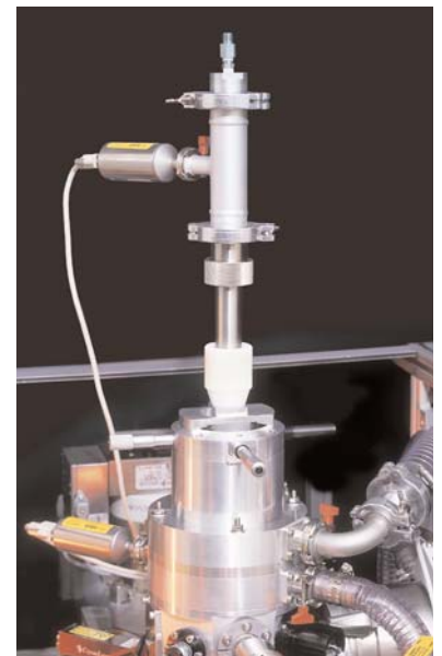
The Aerodynamic Focusing Lens mounts on the ATOFMS inlet.
