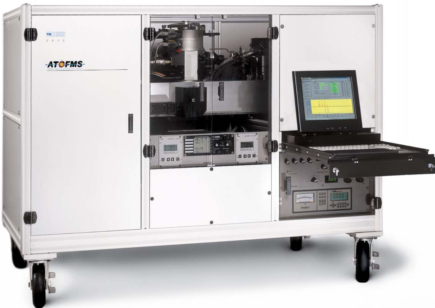
ATOFMS shown without Aerodynamic Focusing Lens installed
