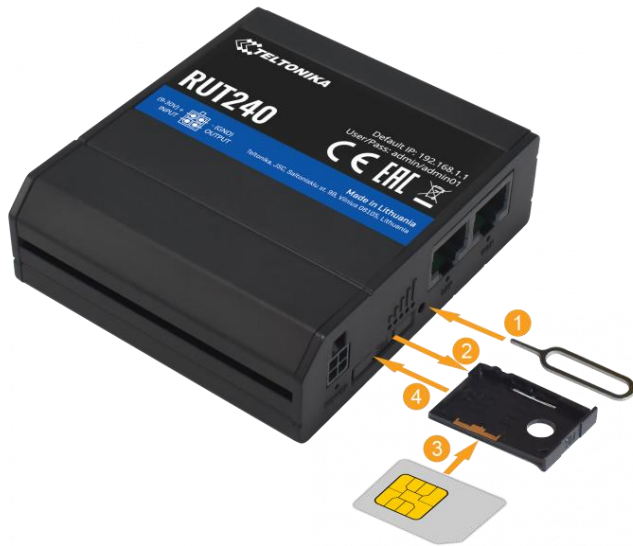
Figure 10: Installation of SIM card
