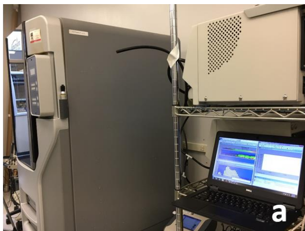
Figure 1: a) The 3D printer (left) with the particle measurement instruments' sampling line positioned in the breathing space outside of the printer. b) Sampling schematic showing the instruments used to measure particles in the worker's breathing space during a print, approx. 0.5 m from the printer's exterior wall.
