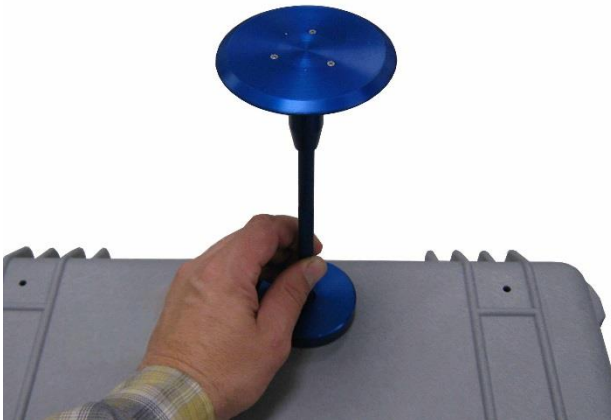
Figure 3: Thread the Inlet into the Inlet Ring
