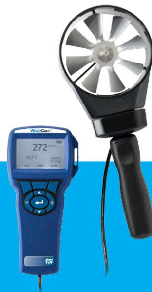
The VelociCalc® 5725 is a high performance, yet simple to use, rotating vane anemometer. High accuracy and reliability make the VelociCalc 5725 the professional's ideal tool for measuring unevenly distributed or fluctuating flows through heating and cooling coils, grilles, and filters.
