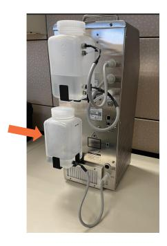
2. Disconnect drain line to water drain, as shown.
