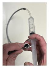
6. Connect the Pump Priming Accessory into the bottom "Water In" sensor port.
