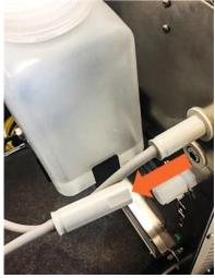
13. Reconnect fill bottle connector to the "Water In" port.
