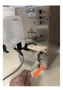
3. Connect Pump Priming syringe (empty of water and with plunger fully inserted) to the **Water Drain** connection on the 9001 lower back panel.
