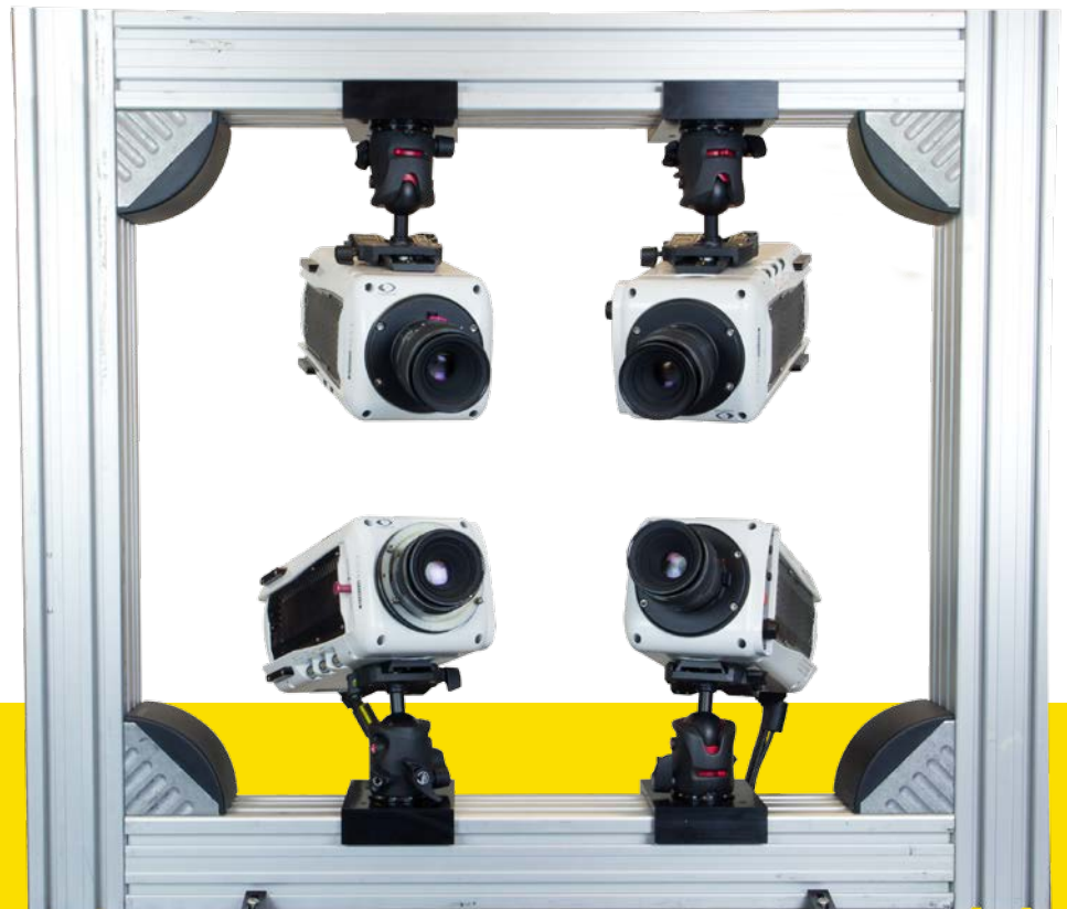
V3V Flex system based on 4-camera configuration
