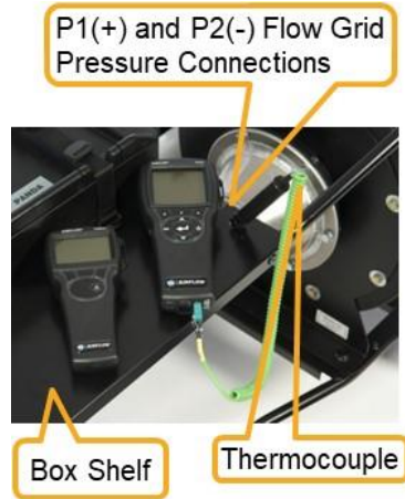
Figure 10. Connecting Instruments to PANDA Tester in High Flow Mode
