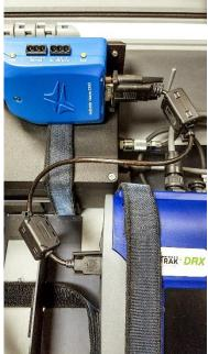
6. Connect the barrel end of the power cable to the DustTrak monitor and the black Phoenix connector to the modem. The third connector is for the heated inlet control module. If the heated inlet is not present, it can left unplugged.
