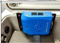
5. Using the RS-232 to USB cable, make a connection between the DustTrak monitor and the modem. The USB end should connect to the DustTrak monitor. The RS-232 end should connect to the modem.
