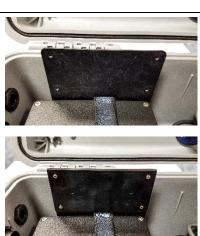
2. Remove the mounting plate from the back of the modem. To separate the two pieces, push the button on the top of the modem, rotate the plate slightly away and slide the mounting plate downwards.
