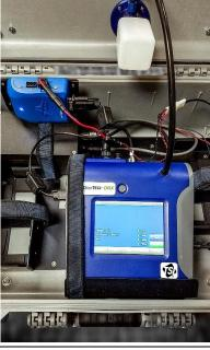
9. LED on the modem will blink while the modem searches for a network. If the LED stops blinking and is solid blue, a network has been found and proper communication with Environet should be possible. If the LED changes to solid yellow, the modem has not found a network. A power cycle may resolve the issue.
