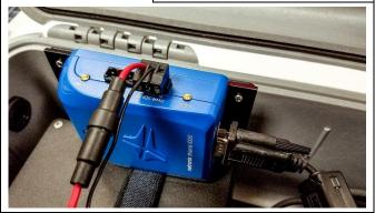
Connect the other end to the power cable to the power source. Same connection will be made if using the solar power system accessory, instead of the 12V DC power adapter.
