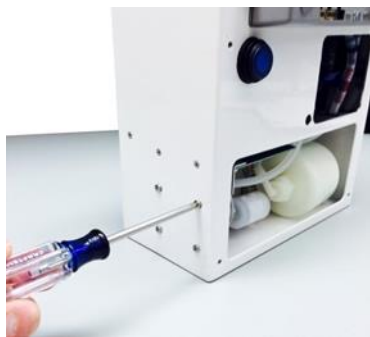
Figure 27: Remove screws from left side panel
