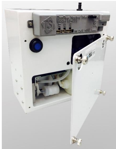
Figure 26: Open instrument service panel
