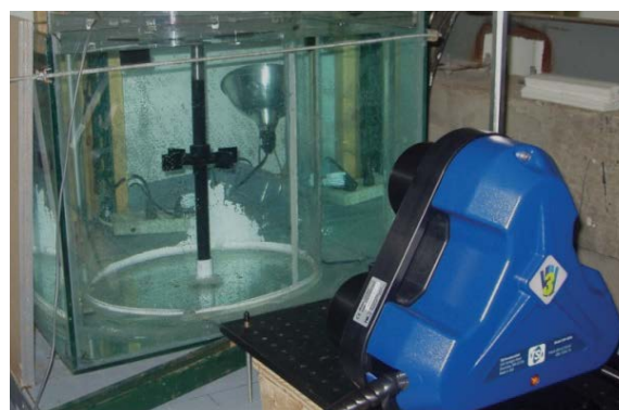
Experimental setup showing V3V™ system camera and Rushton Turbine.
