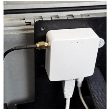
12. Connect the USB cable and RJ45 cable to the DustTrak instrument.
