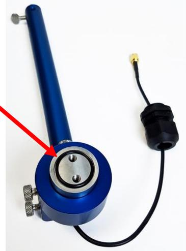
4. Remove the outer most nut on the gland seal.
