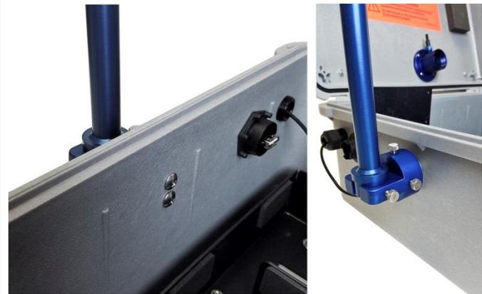
6. Using the nut that was removed in Step 4, attach the gland seal to the side of the enclosure. If needed, use an adjustable wrench to apply a small amount additional of torque to the nut.
