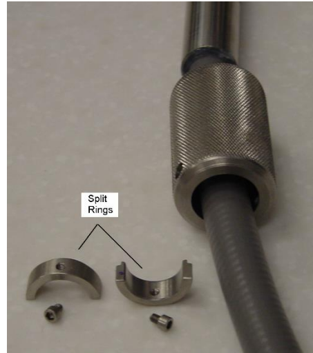
Figure 2. Probe retainer cap installation
