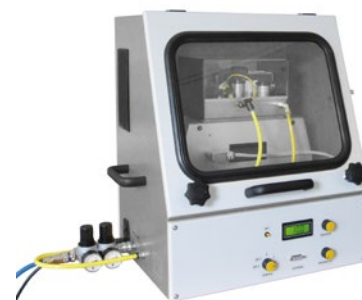
Model 3413U: Dust aerosol generator inside full enclosure for difficult powders
