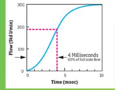
Fast 4 millisecond response ensures accuracy in fluctuating flows. This fast response is ideal for closed-loop control systems and integrated volume measurements. Pressure and temperature measurements are
