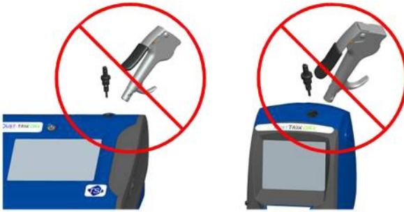
Figure 4-3: DO NOT Blow into Instrument
