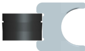
Figure 4-20: Replace Filter Mesh in Filter Holder
