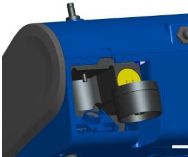
Figure 4-8: Remove 37-mm Filter Cassette
