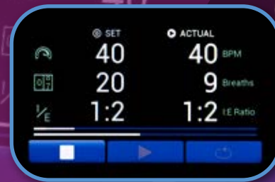
Set v Actual test parameters (during test run, with test progress bar and enhanced visualisation of breath status)
