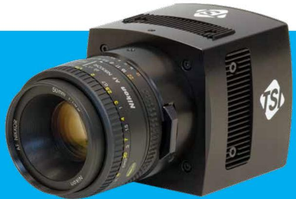
The camera is designed with a defective/hot pixel correction dynamically to ensure all the pixels are used for your imaging requirement to get the accurate flow measurements. Other features, such as short frame straddling times and high quantum efficiency, make it appropriate for a wide variety of applications ranging from hypersonic to creeping flows. The 6MP camera is fitted with an F-mount lens mount and comes standard with a Nikon® 50-mm lens, camera interface and all interface cables.
