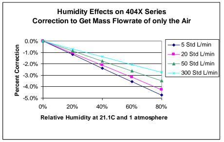
Use the following graph if you are interested in measuring the total mass flow including the water vapor mass.
