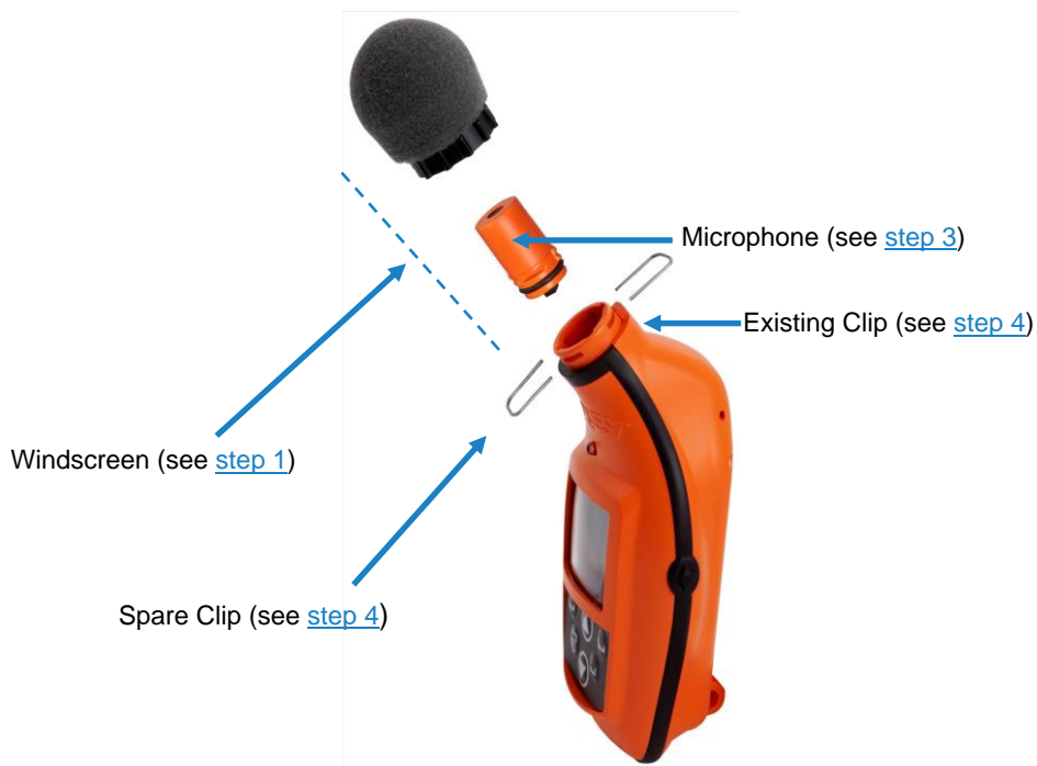
Figure 6-1: Microphone and windscreen assembly
