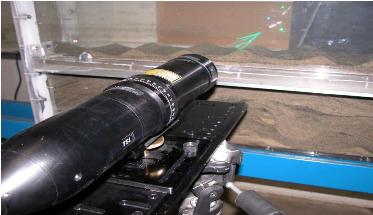
Figure 1: TR260 transceiver probe being used to measure phase-resolved velocities in a water channel flow. (water channel courtesy of the Ven Te Chow Hydrosystems Laboratory at the University of Illinois – Urbana Champaign)
