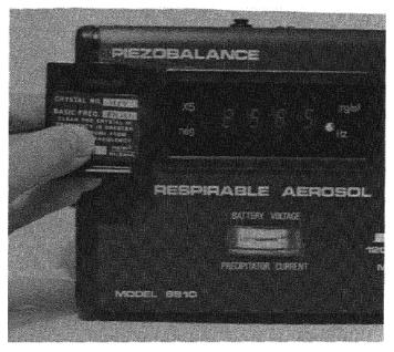
Figure 16. Comparing the sensor frequency with the Basic Frequency.
