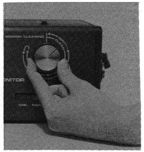
Figure 24. The sensor in the drying position
