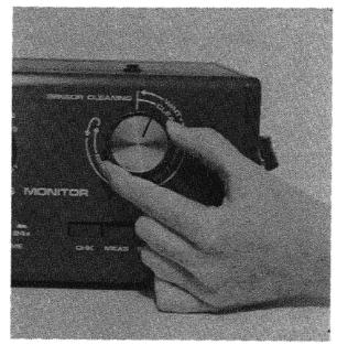
**Step 1.** Turn the Sensor-cleaning dial 10 degrees (Figure 25).
