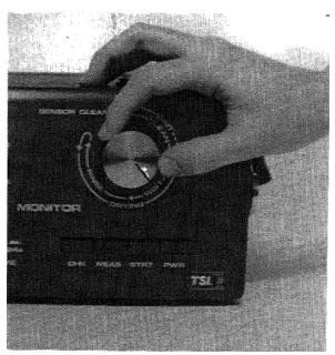
Figure 23. Sensor in the soak position
