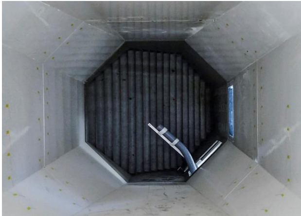
Figure 4. The micro-bubble generator positioned for seeding the wind-tunnel
