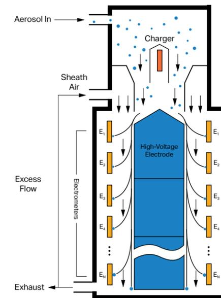
Figure 3. EEPS™ Flow Schematic
