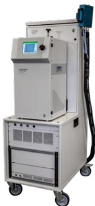
The model 3095 Engine Exhaust Particle Measurement System (EPPMS) is a turn-key emissions measurement solution that combines the 3090 EEPS™ and the 3098 Porous Tube Thermodiluter (PTT). The model 3098 consists of two porous tube diluters (hot first stage and room-temperature second stage) and a catalytic stripper to remove volatiles. The system is fully characterized for losses and is controlled from the EEPS™ software for a seamless user experience.
