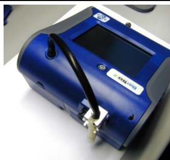
TSI DustTrak II Aerosol Monitor with Dorr-Oliver Respirable Cyclone
