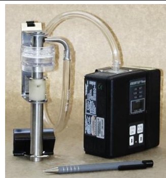
Sample Pump with Respirable Silica Sampling Train
