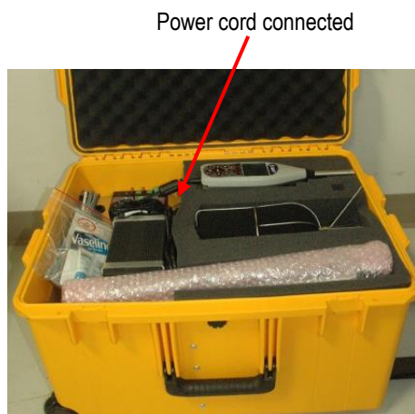
Figure 2: Connecting the battery power
