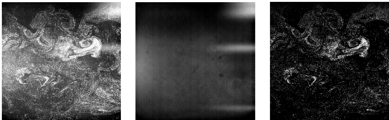
Fig. 4. Benefit of image background subtraction. The images shown are the original image (left), background image (center), and background-subtracted image (right).
