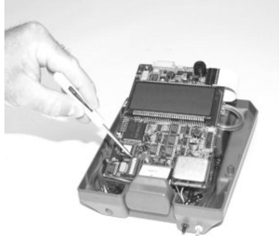
There are 8 DIP switches. The top switch is number 1 and the bottom switch is number 8. A switch is considered to be "ON" when the right side is pushed down and "OFF" when the left side is down.
