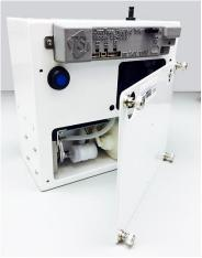
2. Remove the four (4) Phillips-head screws from the left side panel.
