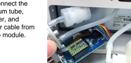
5. Obtain replacement pump. Connect muffler to (P), vacuum tube to (V), and power cable.
