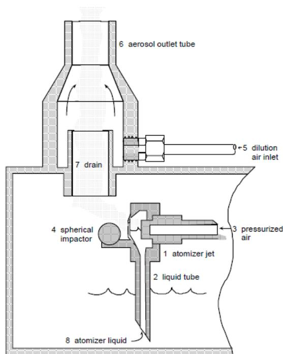
**Figure 2: Schematic of the Atomizer**
