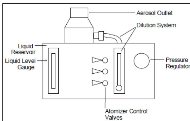
Figure 1: The Four Subassemblies of the Atomizer
