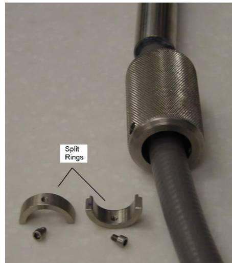
Figure 2. Probe retainer cap installation
