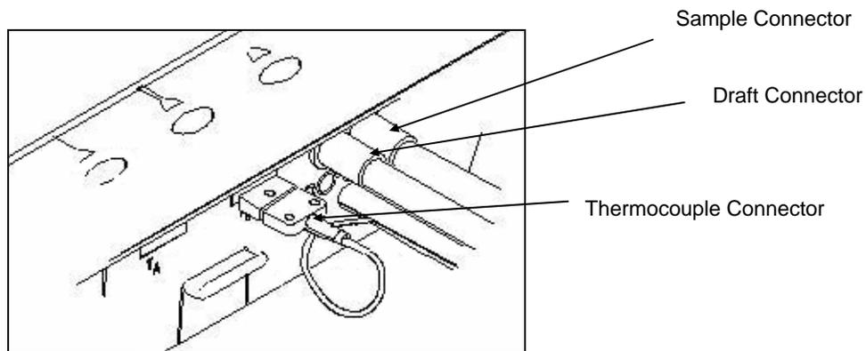
**Figure 3: Sampling Probe Connection**
