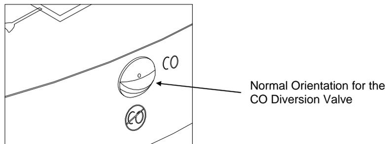
Figure 4: Normal CO Diversion Valve Orientation
