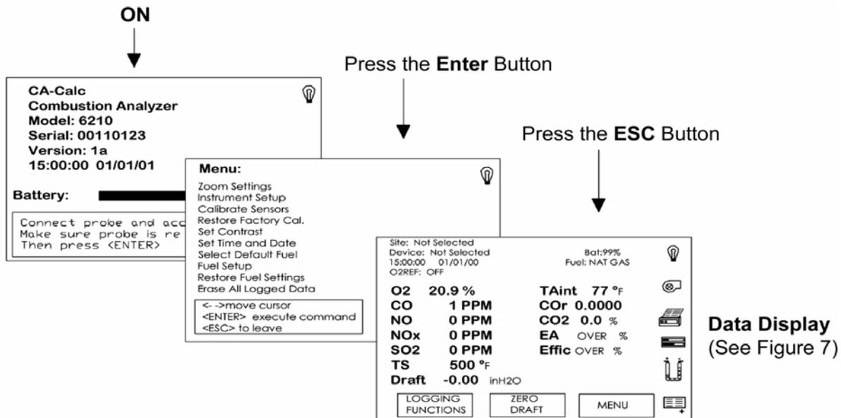
Figure 5: Schematic Illustration of Quick Start Process
