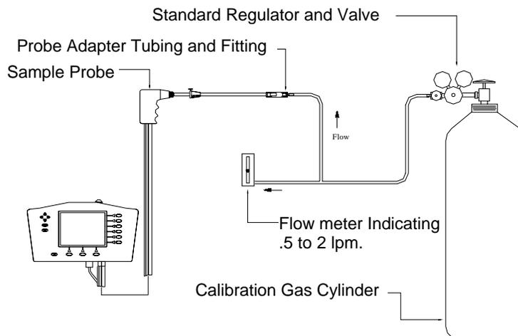
**Figure 18: Alternative Calibration Setup**
