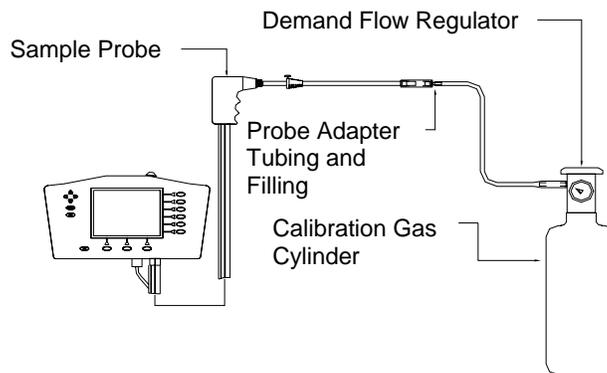
**Figure 17: Calibration Setup Using TSI Calibration Kit Accessories**
