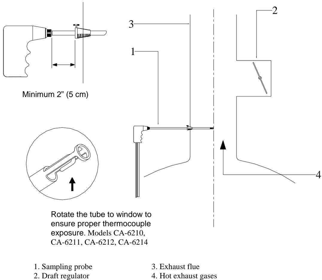
**Figure 7: Sampling Probe Location**
