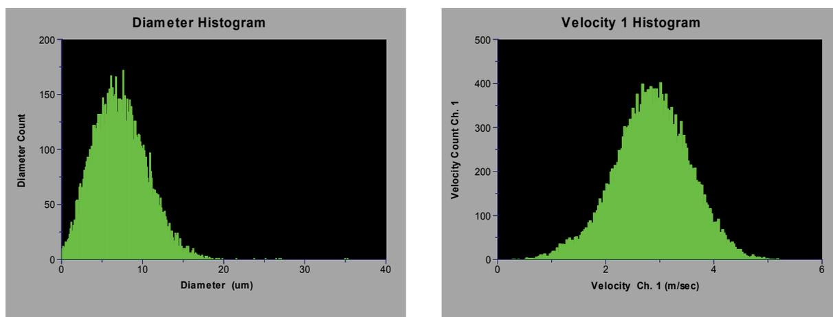
**Figure 1:** Measured diameter and velocity histograms for the entire spray process. Measurements were made on the plume centerline, 25mm from the MDI outlet.
