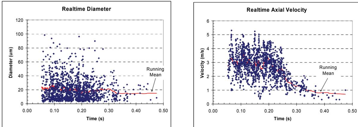
**Figure 2:** Measured transient diameter velocity in the MDI plume. Running mean values are indicated by the (red) line. Measurements were made on the plume centerline, 25 mm from the MDI outlet.
