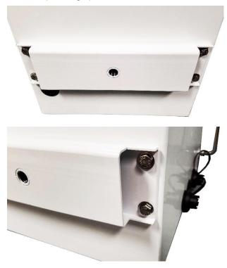
4. Install the instrument onto a surveying tripod. Mount comes with 5/8" - 11 threads to mate with most surveyors tripods.
