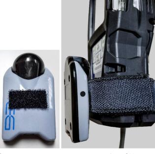
7. Connect the sample probe to the top of the GM460.
