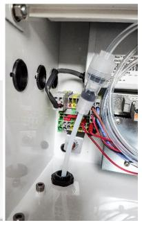
4. Remove the current Li-Ion or Alkaline battery pack from the instrument and attach the continuous operation battery pack. This will allow the GM460 to operate continuously, as long as the environmental enclosure has power.
