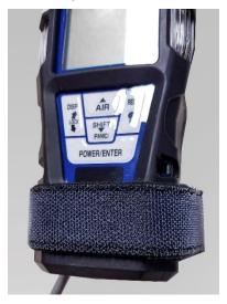
6. Apply the small piece of Velcro® with adhesive back to the IrDA reader and attach it to the front of the GM460.
