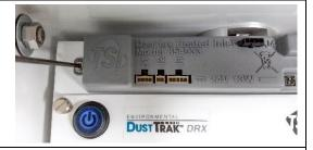
Push out elastic plug and install RH/Temp Sensor sealing gland. Removable nut should be installed on the inside of the enclosure.
