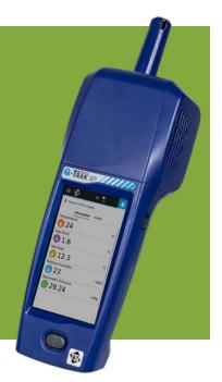
The Q-Trak<sup>™</sup> XP Indoor Air Quality Monitor Model 7585 combines multiple gas and particle measurements into a single lightweight, handheld instrument that is easy to use, configure and calibrate in the field.
