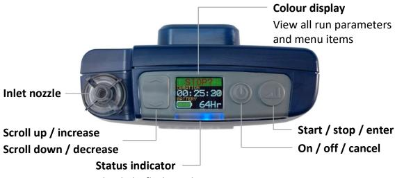
Blue light flashes when pump running Red light flashes when there is a fault or during charging
