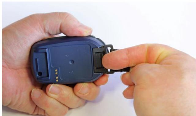
Should the clip assembly require replacement, hold the dBadge2 with the back uppermost in one hand and with the other hand simultaneously lift the tab with a finger whilst pulling the clip away from the dBadge2 body. There is a knack to this operation to deter tampering. A pack of spare clips (5 pairs) is available (part number DB2CLIPS). When refitting the clip assembly ensure that the tab is locked by pushing it into place and pull on the clip assembly to check that it is secured.
