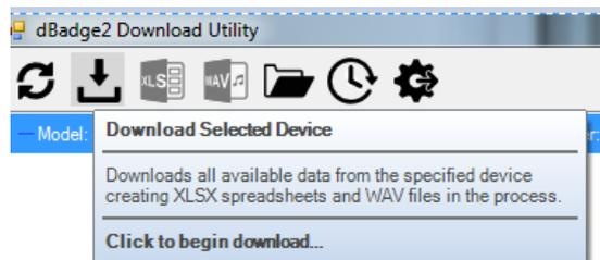
With the dBadge2 to be downloaded in the left most 'pocket' of the Docking Station, powered and connected by the USB cable, click on the icon as shown below to search for connected devices
