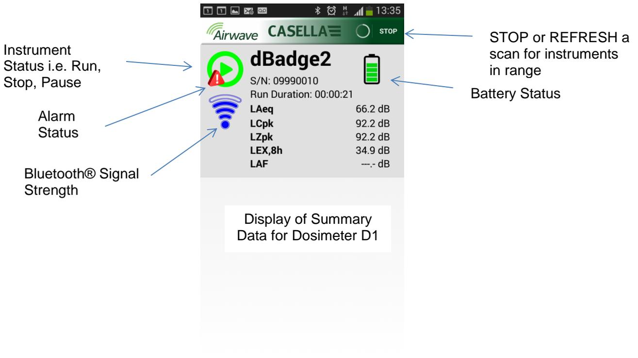
To save power, the Airwave App stops scanning once all instruments within range have been detected. To scan for new instruments, press 'REFRESH' in the top right corner of the mobile device display.
