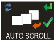
If selected the display will automatically scroll from one screen to the next (otherwise the screen has to be advanced manually). Press the right 'R' key to accept or left 'L' key to change
