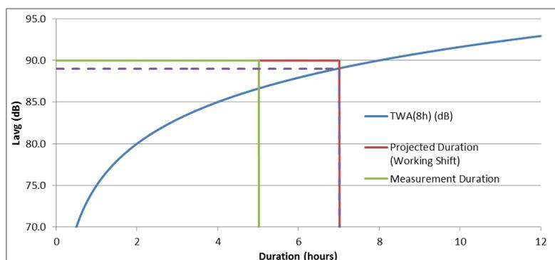
**Figure 4 shows a measurement of 5 hours (green line); this is then projected forward to the end of the 7 hour working shift (red line); where the projected value crosses the original TWA(8h) (blue line) is the actual TWA(8h), shown by the dashed line. (NOTE this is based on using levels of 90 dB and are only for illustration. In practice the TWA(8h) would be calculated mathematically from the Lavg at the end of the projected 7 hour working shift)**
