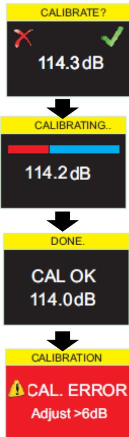
Press the right 'R' key to confirm you wish to calibrate, or the left 'L' key to cancel the operation. It will take a few seconds to automatically calibrate to 114 dB during which time a progress bar is displayed as shown.
