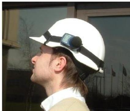
It is also possible to attach the dBadge2 to a harness (part number D8147/Z) by feeding the harness through the blank webbing buckle clip fittings (part number 207073B). For any existing harness that an employee might already be wearing, use the pin attachment. In addition, the
