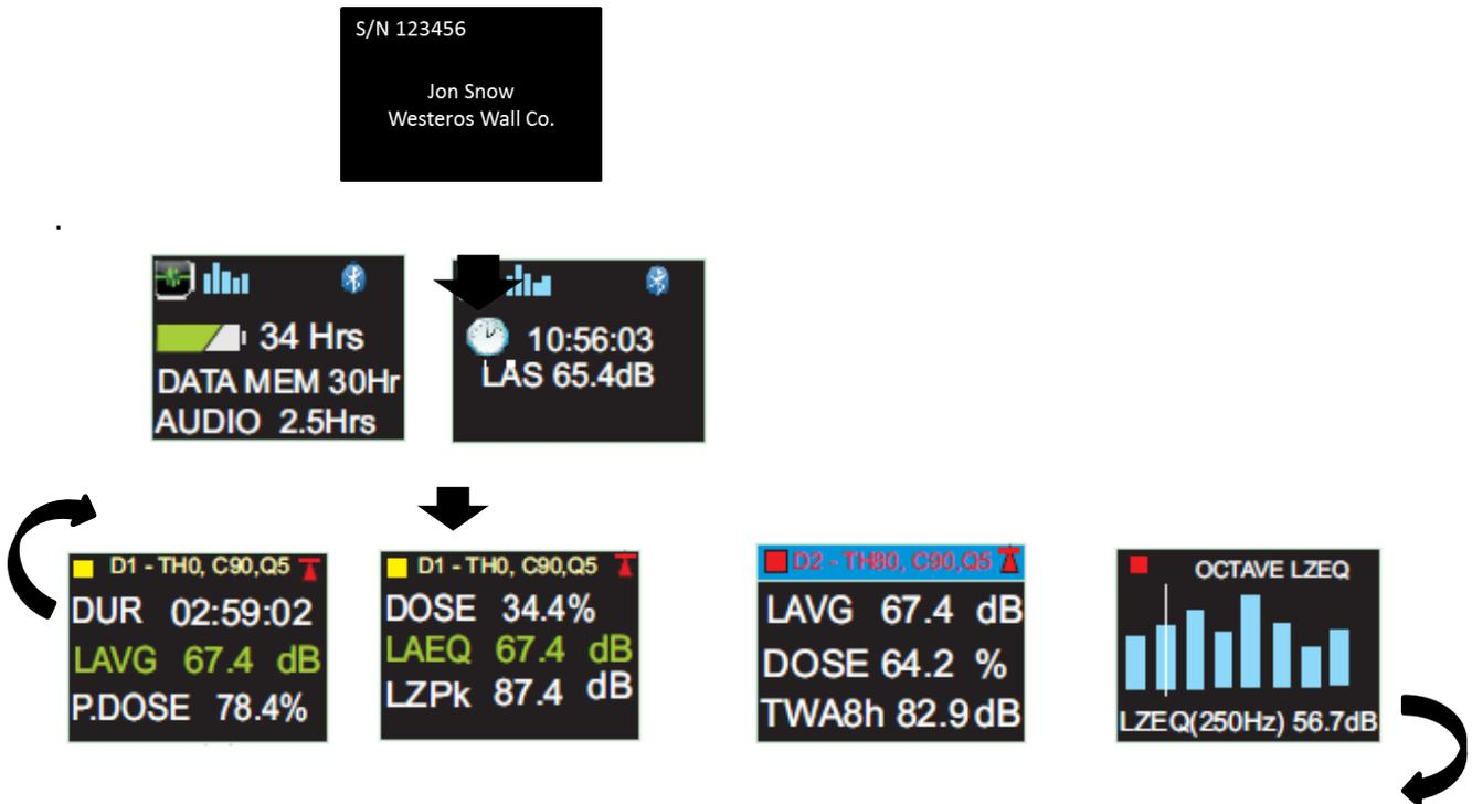
If the Autoscroll feature has been disabled (see Section 7.14) pressing the right 'R' key will scroll through the available results from the last run depending upon how the dBadge2 was configured e.g. octave band results are shown above, which are only available on the Pro model and if selected in the configuration menu (see Section 7.8).
