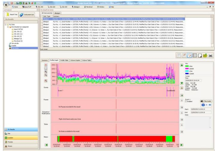
A colour coded system can be used to highlight workers who have been exposed to specific action levels. Graphs can be modified by adding exclusion zones, which subsequently provides exposure data with and without these zones. Data can also be viewed according to different measurement protocols e.g. either ISO or OSHA or alternatively the data can be customised to a user's own requirements.
