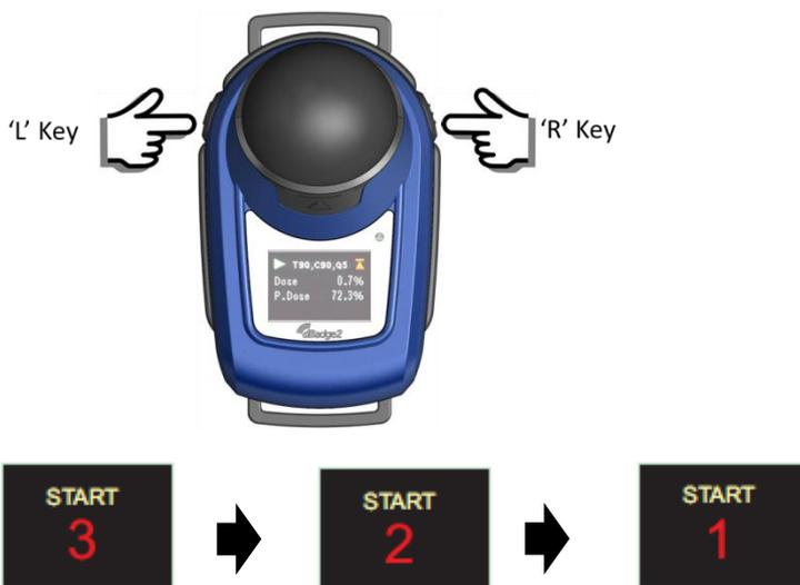
The keys must remain depressed during the countdown for the measurement run to begin; releasing during the 3-2-1 countdown will cease the operation.
