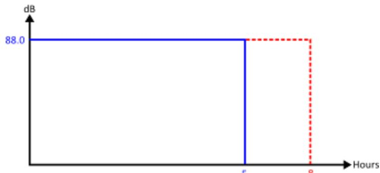
Figure 7 shows the 5 hour measurement (blue line); but also the same noise level continued for the rest of the 8 hour shift (red line)
