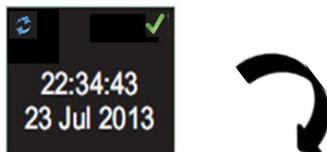
If the data and time are correct, press the right 'R' key to advance to the next menu option otherwise press the left 'L' key to make adjustments. The value to adjust will highlight in red.
