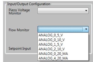
Figure 34: Flow Monitor Configuration
