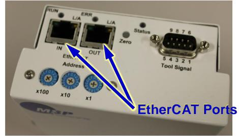
Figure 10: Location of EtherCAT Ports
