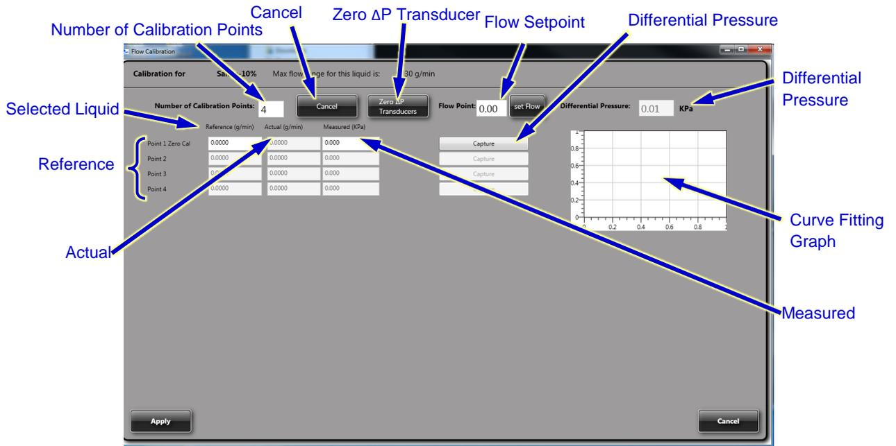
Figure 44: Calibrating a Liquid using a 'New Calibration' method
