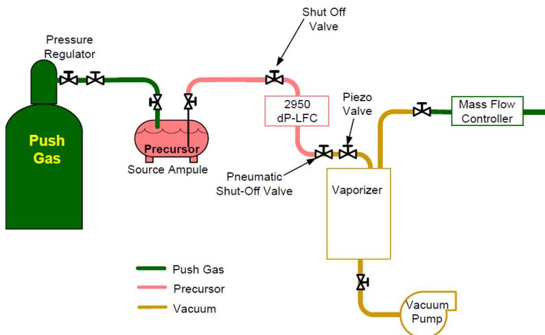
Figure 12: Priming the 2950 LFC
