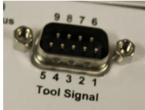
Figure 31: Tool Signal Pinout
