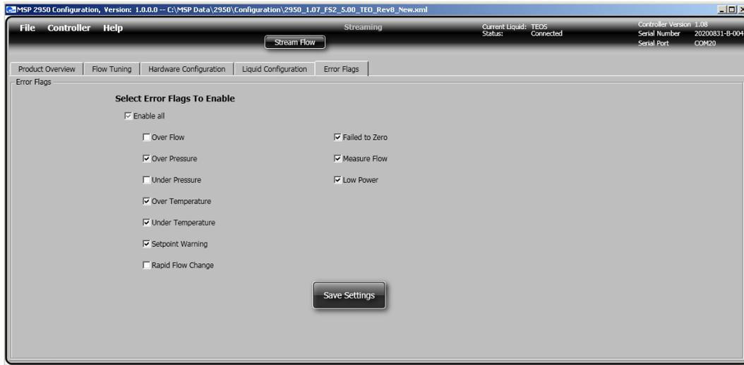
Figure 47: Setting Error Flags on the Error Flags tab
