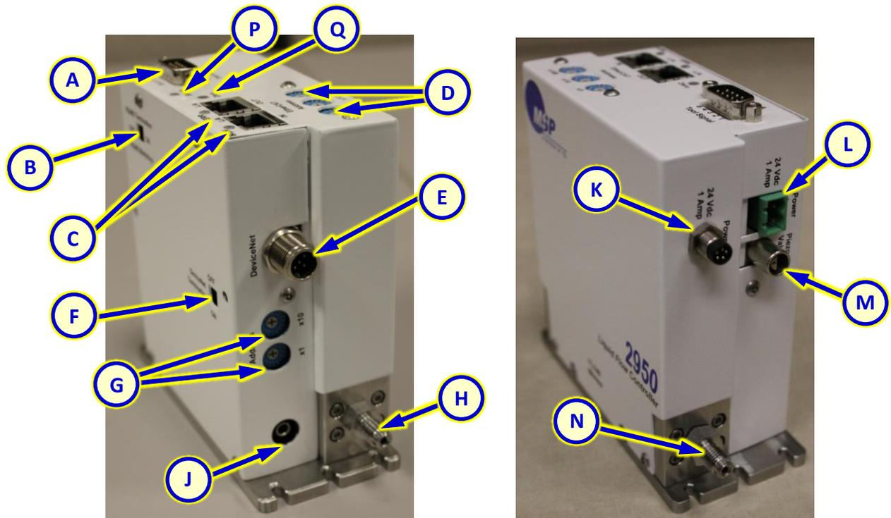
Figure 2: Connectors, Switches & Ports on the LFC
