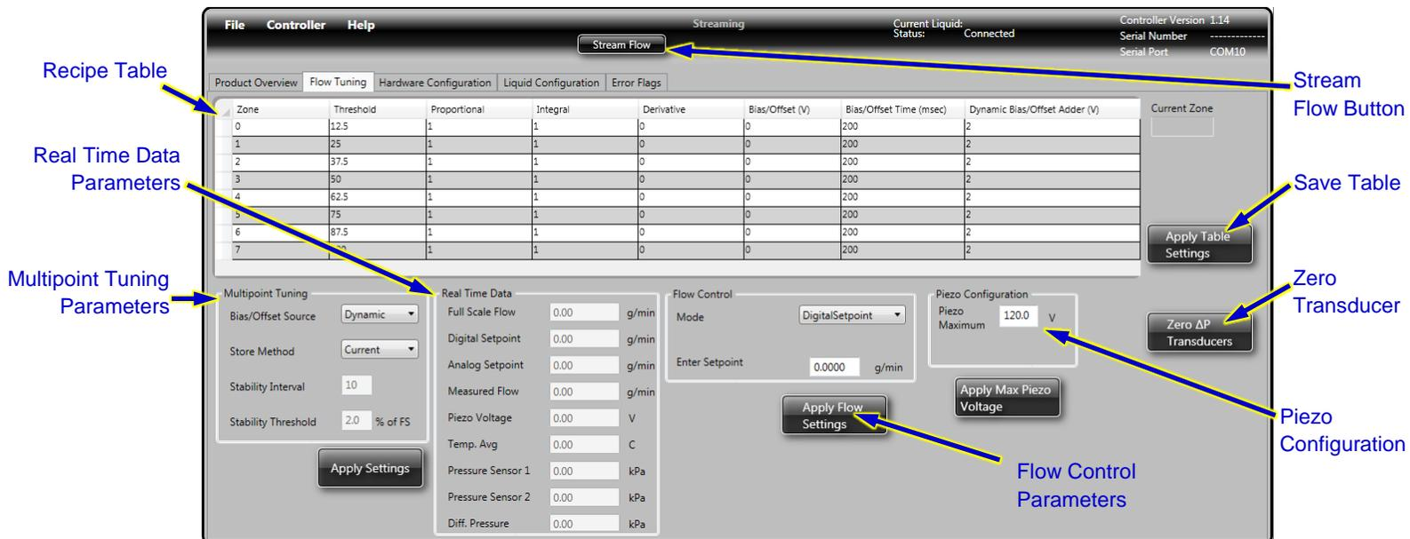
Figure 18: Flow Tuning Tab
