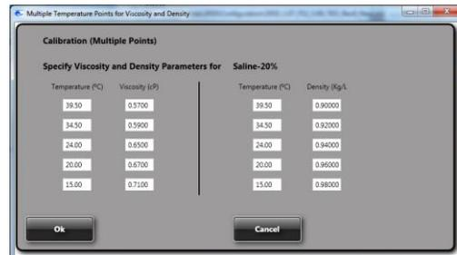
Figure 43: Entering Dynamic Temperature parameters for a New Calibration
