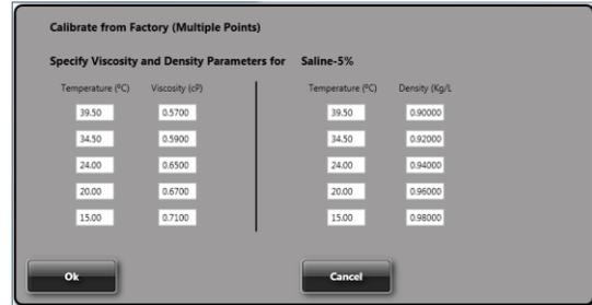
Figure 42: Calibrating a Liquid using a Factory Liquid using Dynamic Temperature
