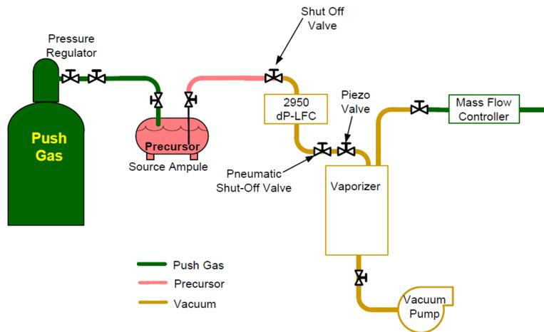
Figure 11: Evacuating the 2950LFC
