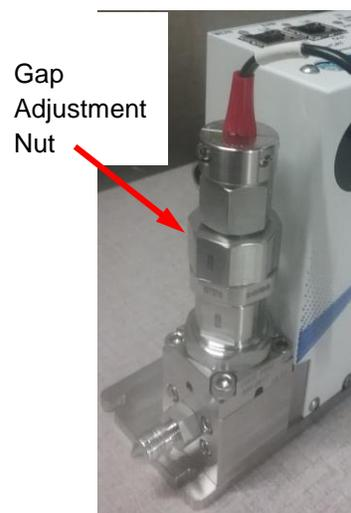
Figure 2 • Adjusting the Piezo Valve Gap
