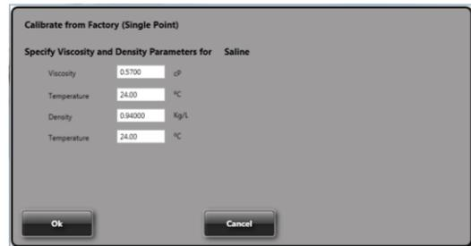
Figure 41: Calibrating a Liquid using a Factory Liquid using Static Temperature
