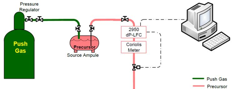
Figure 40: Calibrating 2950 LFC using a second flowmeter.
