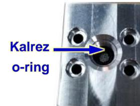
Figure 56: o-ring in place
