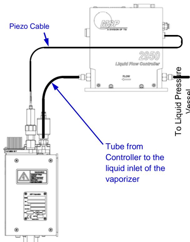
Figure 3: Connecting 2950 to a 28XXPE Vaporizer
