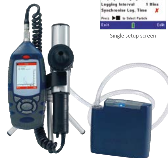
Gravimetric calibration to calibrate for specific dusts
