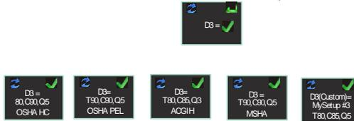
Dosimeters D2 and D3 may be enabled to show additional LAVG based Dose results based upon alternative Threshold, Criterion and Q Factor Exchange rates
