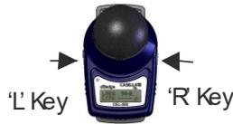
To Enter Configuration Mode, Press L and R Keys Together at Switch On
