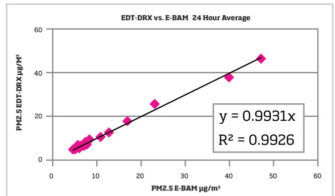
The PM2.5 24-hour average data from the EDT-DRX compares extremely well with the E-BAM (Slope of 0.993 and R² of 0.99), as supported by the correlation plots above.
